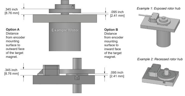
Images show two inch magnet rotor, but alignment targets hold true for all sizes.
